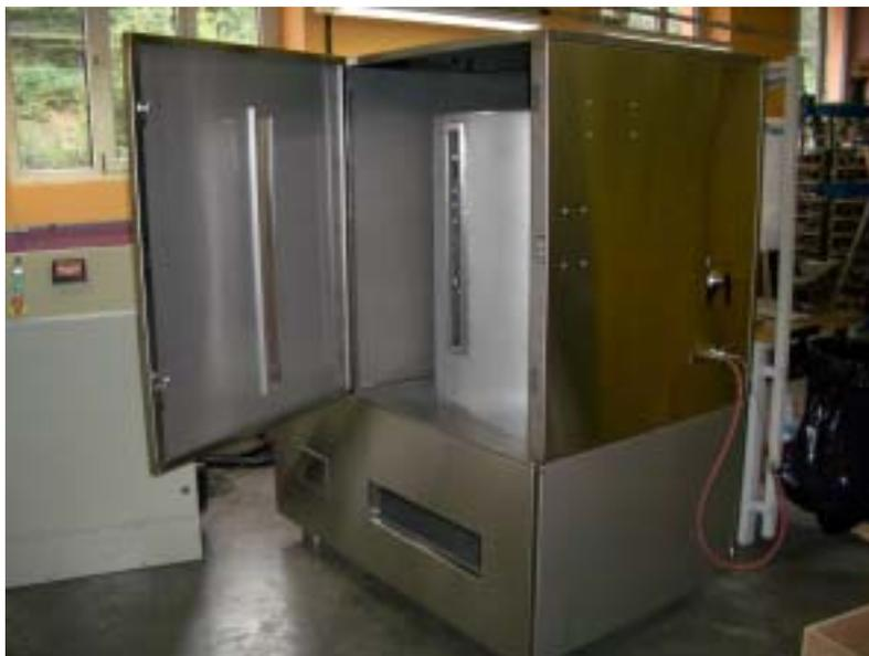
The Partitron 25 CPC (fig. 1) of dimension: 1.50 (L) x 1.00 (D) x 1.85 (H) m; weight: 1,200 kg (see description of the rotor in section Results and discussion) was connected through 2 rotating seals (tungsten carbide, 150 bars; 1,500 rpm) from DEUBLIN (Vaukegan, IL, USA) to:
